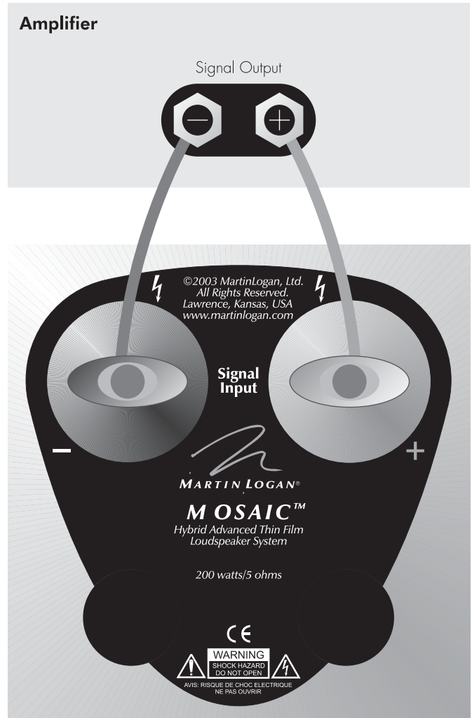
Figure 1. Single wire connection. One channel shown.
