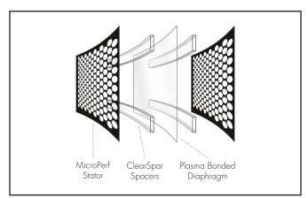
**Figure 14.** Cut away view of an XStat<sup>™</sup> electrostatic transducer. Notice the simplicity due to minimal parts usage.
