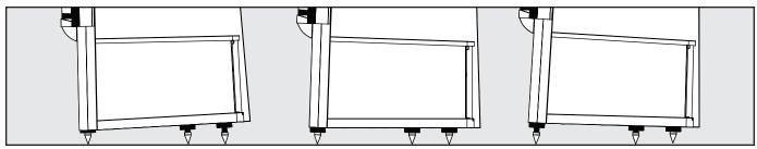
Figure 6. Adjust rake of the CLX by varying the height of the jam nut, and/or by removing the jam nut.
