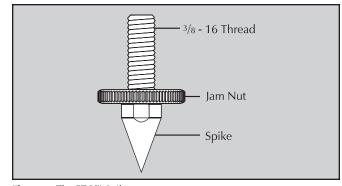
**Figure 5.** The ETC<sup>™</sup> Spike.
