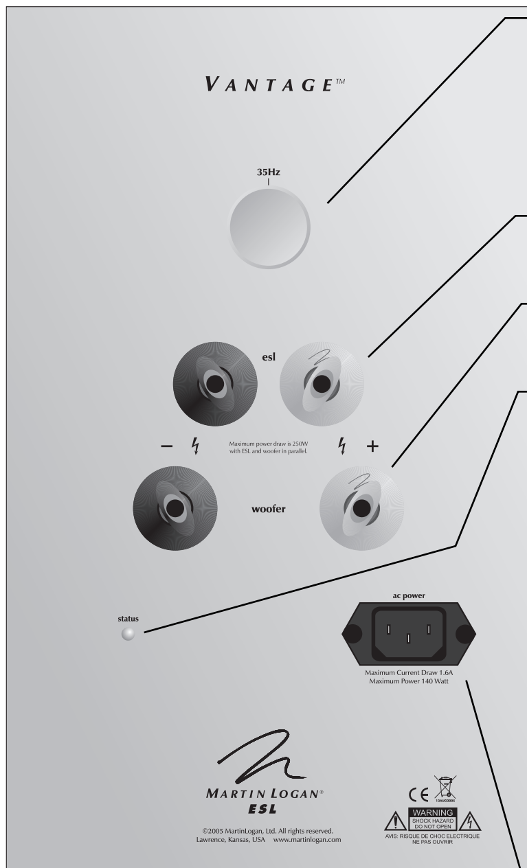
Figure 1. Vantage Controls and Connections
