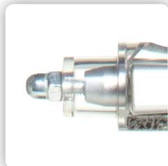
A robust mounting-lock system allows quick, trouble-free installation. When not in use, the constant-control mounting locks are held securely within a self-contained housing. When moved into place during installation, they couple the speaker's chassis firmly to the ceiling. And if the speaker is ever removed, the locks retract and latch themselves back in their housings.
