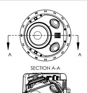
33° TWEETER AIMING: ROTATE SPEAKER ASSEMBLY TO AIM TWEETER AT LISTENING POSITION
