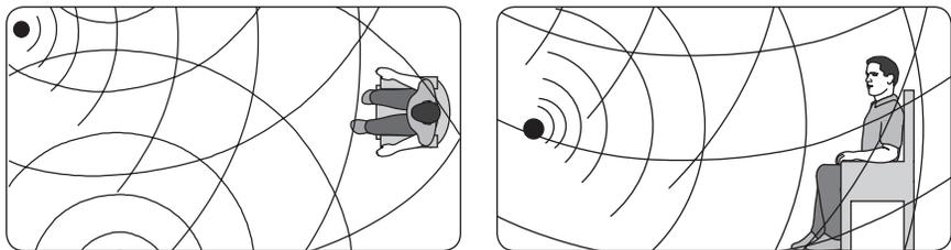
**Figure 16–17.** Even though they suffer from “venetian blind” effect, angled multiple panel speakers can deliver good imaging, but only to specific spots in the listening area.
