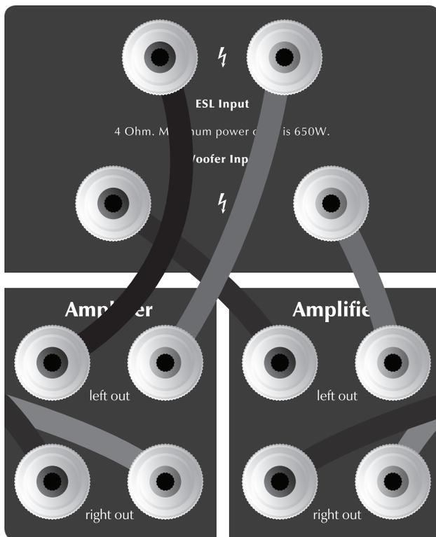
**Figure 4.** Horizontal passive bi-amplification. One channel shown.
