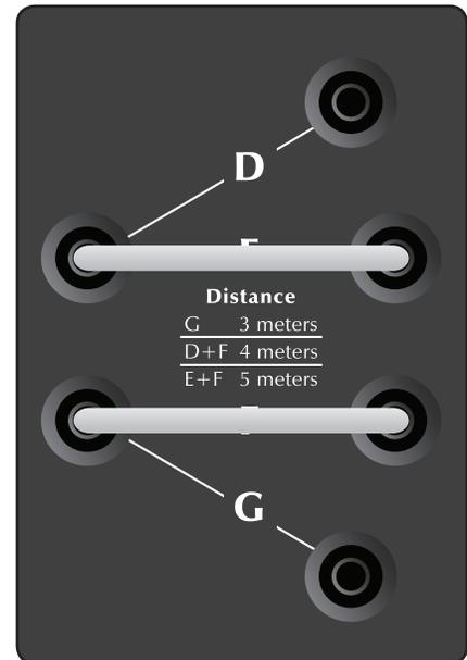
Figure 9c. Distance jumpers set for 5 meters.
