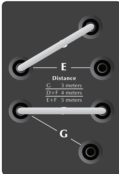
Figure 9b. Distance jumpers set for 4 meters.
