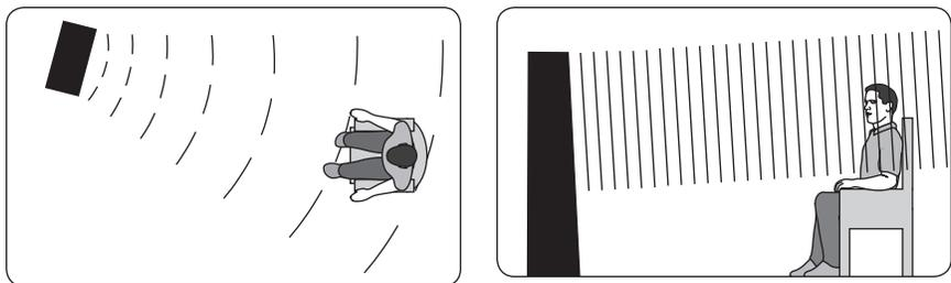
**Figure 18–19.** A controlled 30 degree cylindrical wave-front, a MartinLogan exclusive, offers optimal sound distribution with minimal room interaction. The result is solid imaging with a wide listening area.
