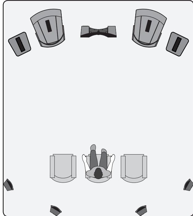
**Figure 20.** Neolith speakers as front channels, MartinLogan electrostatic speakers as center channel and rear and side surround (effects) channels, and MartinLogan subwoofers as LFE (effects) channel.
