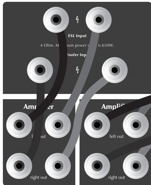
**Figure 5.** Vertical passive bi-amplification. One channel shown.
