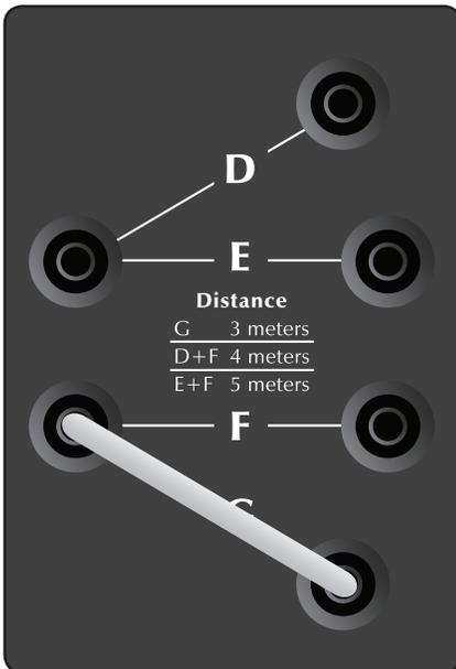
Figure 9a. Distance jumpers set for 3 meters.
