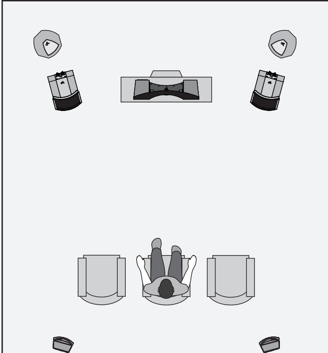
Figure 11. Summit XJR speakers as front channels, MartinLogan electrostatic speakers as center and surround (effects) channels, and MartinLogan subwoofers as LFE (effects) channel.
